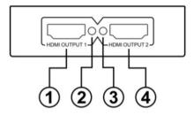
Output 1: This slot is where you connect the HDTV or monitor with HDMI cable.
